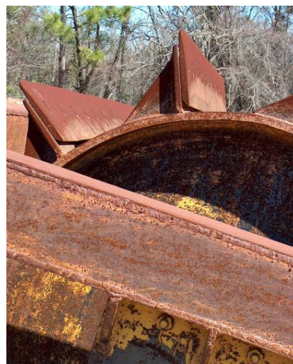
Close-up of drum chopper blades.
